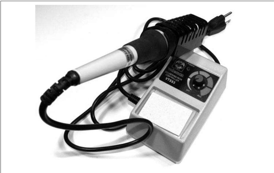
Figure A-19. Soldering station
