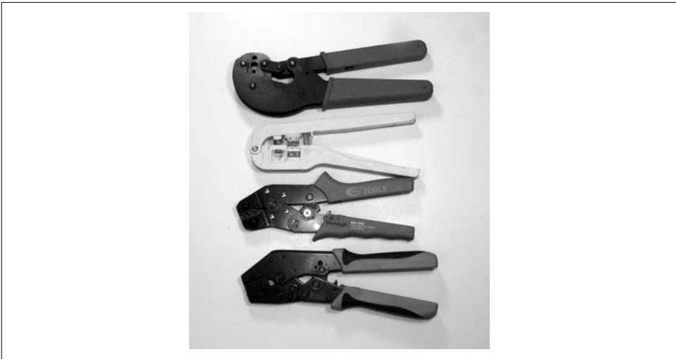
Figure A-8. Various types of low-cost crimping tools
